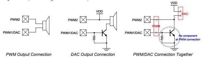
When using the PWM output, we provide an option of normal PWM current or large PWM current for different customer demand. The large PWM consumes more current and makes sound louder.
