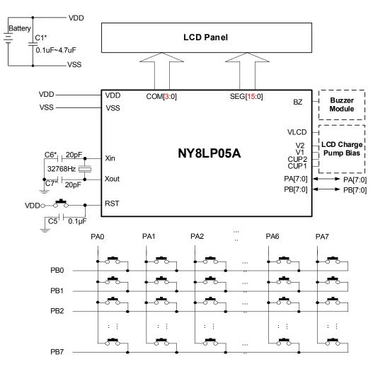
Fig.13-1: The Application Circuits with & LCD
