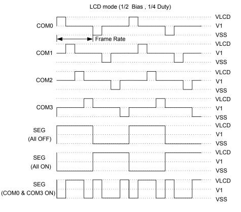
Fig.8-2: LCD timing waveform of 1/2 bias, 1/4 Duty
