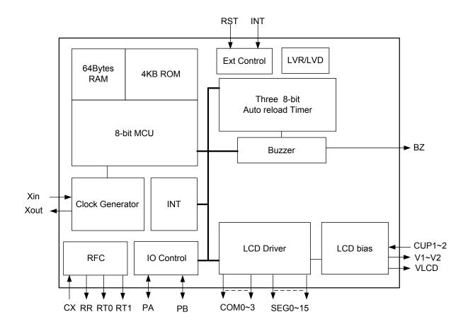
Fig.3-1: The block diagram
