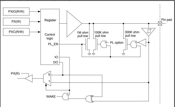
Figure 10-1: I/O port Configuration
