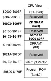
Figure 7-1: The structure of address mapping for NY8LP05A
