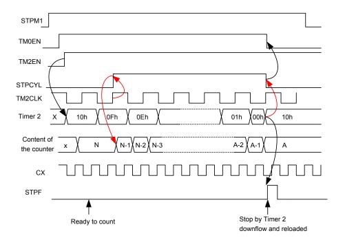
Figure 11-3: Timing of the RFC counter controlled by Timer2 downflow
