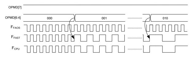
Figure 5-3: The procedure of dividing CPU clock
