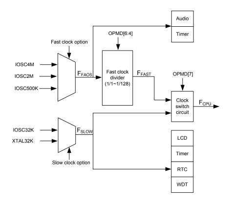
Figure 5-1 Oscillation Configuration
