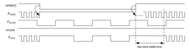
Figure 5-4: The procedure of switching operation modes
