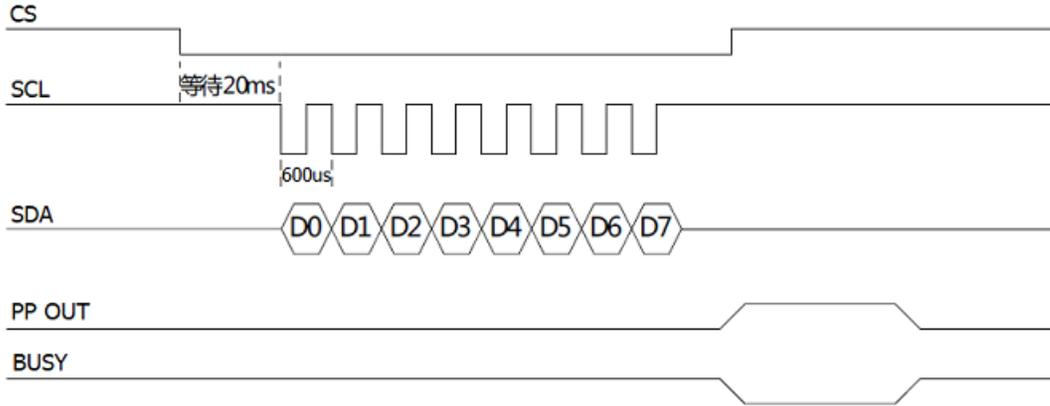
If the reset signal is applied for special industrial products, please notice that IC takes 32ms to restart, then lower SDA to start sending commands. The Busy is output, the playback of audio will output Busy High or Busy Low according to user's setting.
