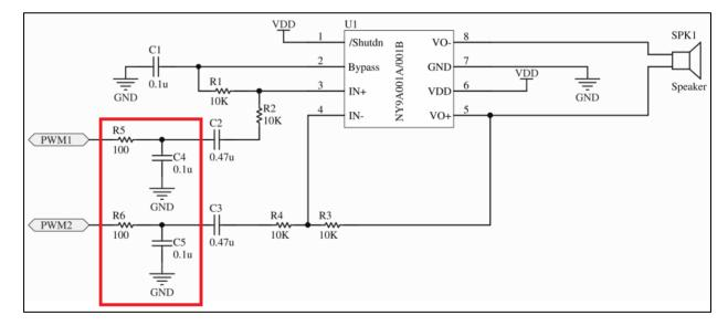
Illustration: Execute the differential amplifier when the PWM signals pass the RC low-pass filter.
