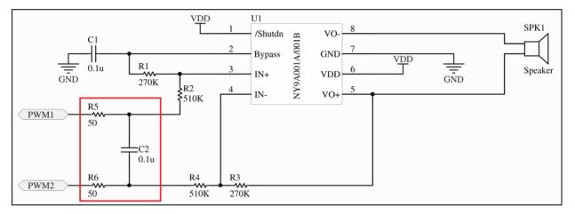
Illustration: Execute the differential amplifier when the PWM signals pass the RC low-pass filter.
